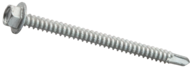
R-LS LARGE FLANGE SELF-DRILL SCREWS For base rail fixing between 25mm – 100mm Steel up to 3.5mm & render board
